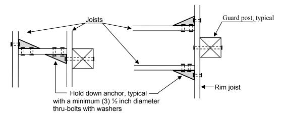
Post can be located on the inside of the joist.
