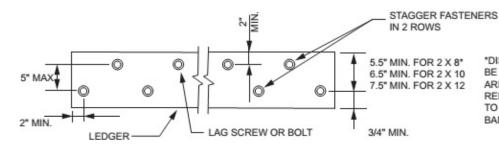
\*DISTANCE SHALL BE PERMITTED TO BE REDUCED TO 4.5" IF LAG SCREWS ARE USED OR BOLT SPACING IS REDUCED TO THAT OF LAG SCREWS TO ATTACH 2 X 8 LEDGERS TO 2 X 8 BAND JOISTS.
