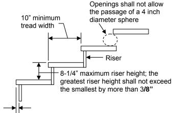
3/4"-1-1/4" nosing; the greatest nosing projection shall not exceed the smallest by more than 3/8"
