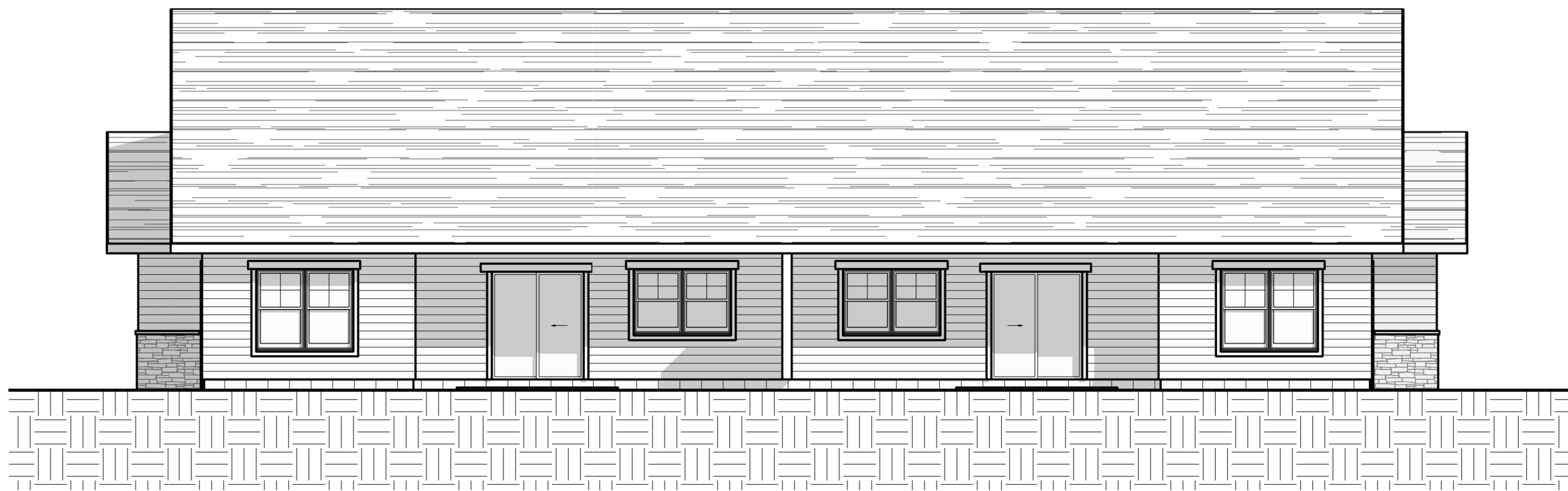
3 2 UNIT - 2-BED RANCH - REAR ELEVATION 1/8" = 1'-0"
